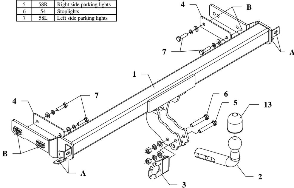
This towing hitch is designed to assembly in following car: **VOLKSWAGEN PASSAT CL, 4 doors, ESTATE**, produced since 10.1993 till 09.1996, catalogue no. **K19** and is prepared to tow trailers max total weight **2000 kg** and max vertical mass **85 kg**.
